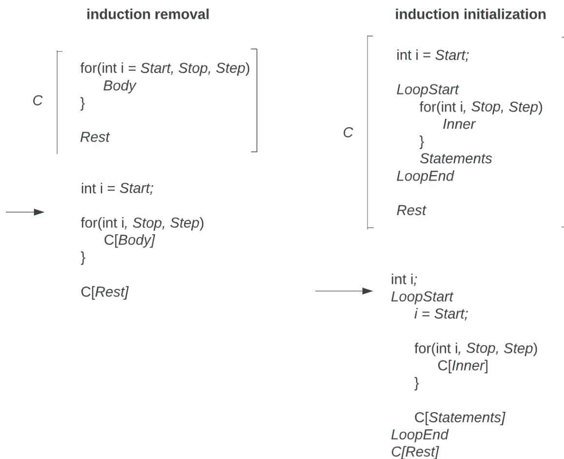
In the induction removal transformation, we extract the start expression into a separate variable declaration and recursively apply this transformation to the body statements and post statements. After extracting the induction variable, we perform an assignment right before the for loop statement for nested loops to ensure that the variable is assigned the start value each time the loop iterates. This helps prevent issues, such as those explained above, from arising.
