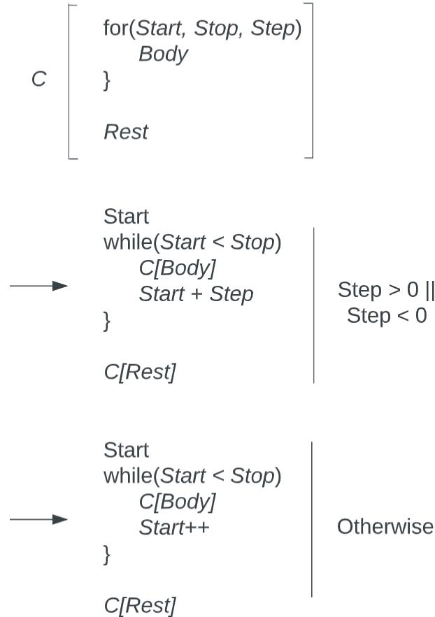
To do this we should take in consideration that a for loop can have a negative step value. This changes the behavior and we quickly figured out that the ternary can be used to encode this logic. This is how we implemented it:
